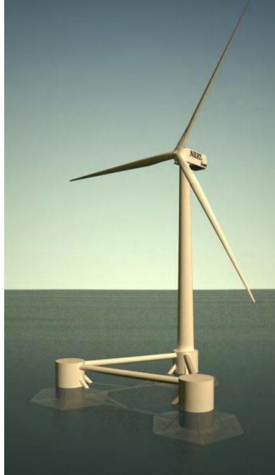
Figure 5.2.1 WindWave semisubmersible platform [29]
